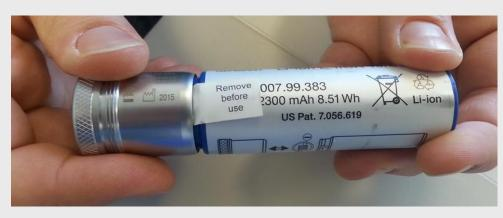
Remove battery completely from handle.
