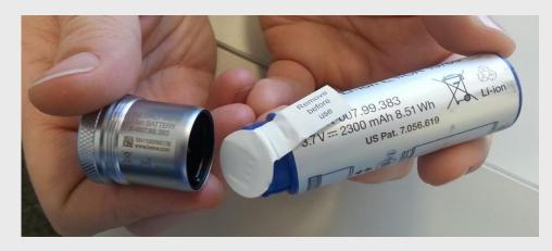
Remove the insulating foil between the bottom cap and the battery
